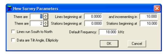
Stations and lines are assumed to be evenly spaced, but this can be changed later. The survey is defined as consisting of a number of lines and a number of stations per line, so the data are laid out on a regular rectangular grid. Specify the number of lines and number of stations per line and the beginning value and increment for each.
