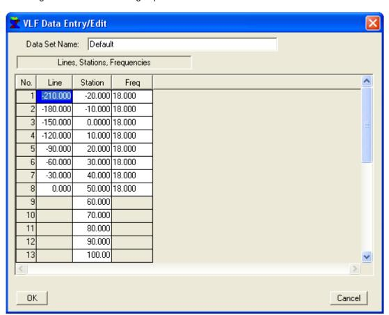
This does not allow you to delete or create additional lines or stations, but it allows you to edit the present values. Stations or lines which are nonexistent are grayed out (read only).
